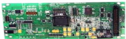
Burner Management System (BMS)
